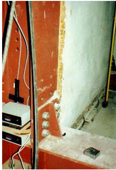
Figure 8: View of electronic display units and end of tape. (Photograph P. Florence)
