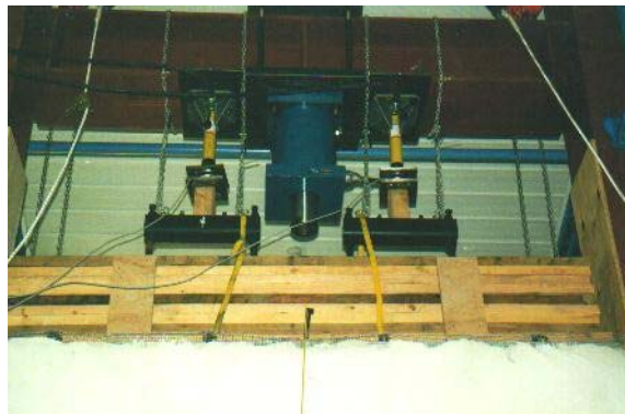
Figure 6: Hydraulic rams and top plate assembly. (Photograph P. Florence)
